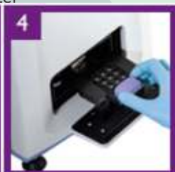
4 Biochip carrier masuk kedalam Evidence
